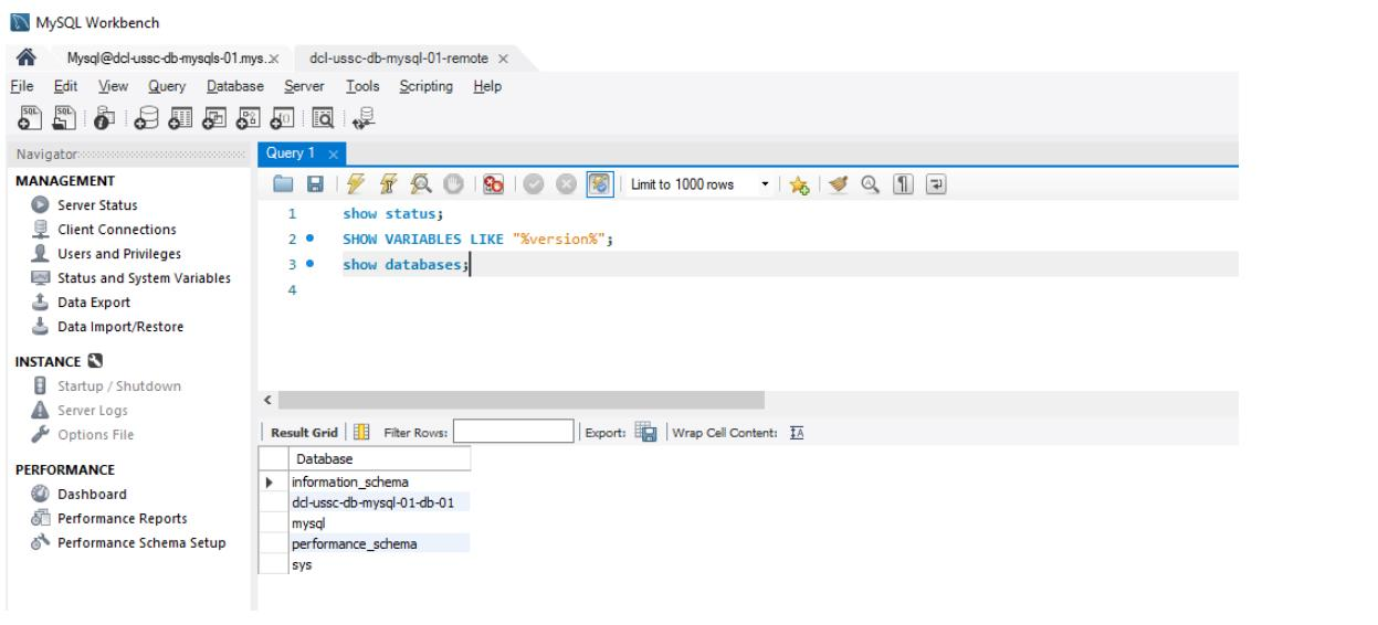
Workbench allows you to open multiple connections either to one or more than one MySQL servers. Each connection shows up in a tab, you can switch from one connection to another by selecting the desired connection tab. This way you may multi-task working with multiple servers at a time.
